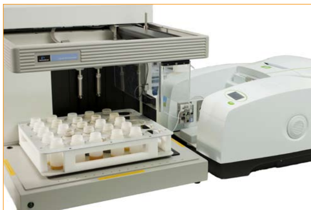
Figure 3. The Frontier OilExpress provides complementary measurement of oil contaminants, oxidation and nitration products.
