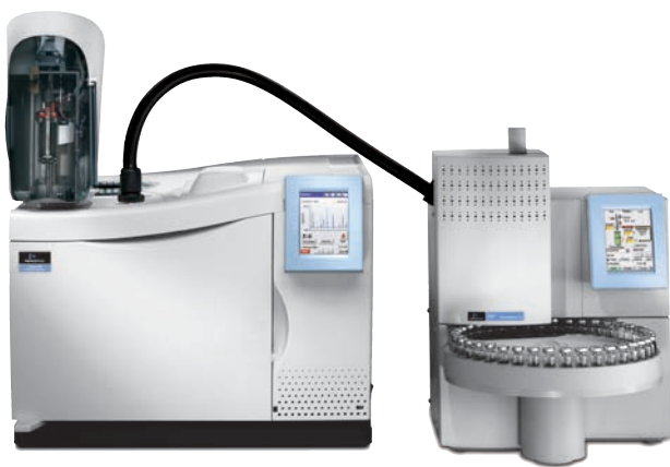
Figure 5. Clarus GC with liquid and headspace autosamplers for simultaneous determination of fuel dilution and glycol contamination.
